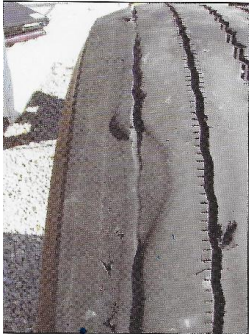
Example of cupping/scallop/wavy wear due primarily to a tire being out of balance.
