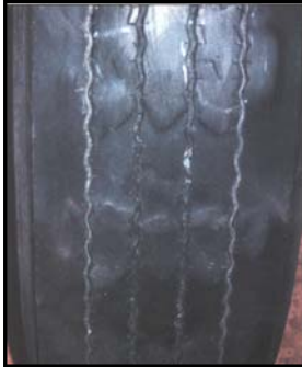
Trailer tire showing signs of irregular wear aggravated by improper inflation
